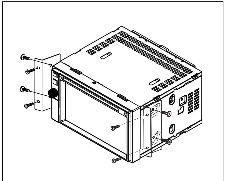
**CAUTION! Do not exceed M5 X 6MM screw size. Longer screws may damage components inside the chassis.**
